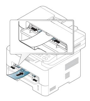
If envelopes are printed out with wrinkles, creases, or black bold lines, open the rear cover and try printing again. Keep the rear cover opened during printing.
